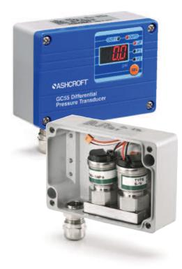
Two sensor DP design means three measurement variables in one device. Output, display and switch settings can be set in nearly ANY independent configuaration to monitor, high pressure port (P1), low pressure (P2), differential (P1-P2).
