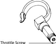
Picture 1 – Bourdon Tube with Throttle Screw Installed
