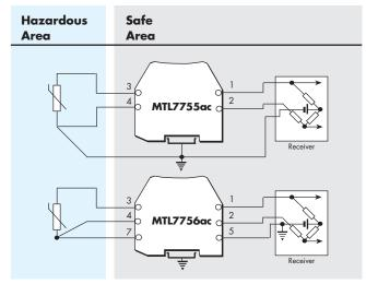
Figure A6: Low-level analogue inputs (RTD's)
