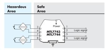
Figure A7: 2-channel switch/proximity input
