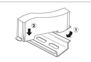
Figure 6: Clamping an MTL7700 Series barrier on to a DIN-rail
