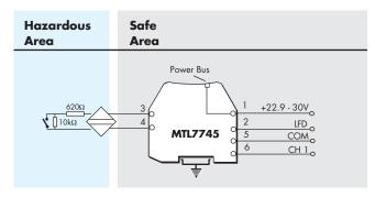
**Figure A10:** Single channel switch/proximity input with Line Fault Detect
