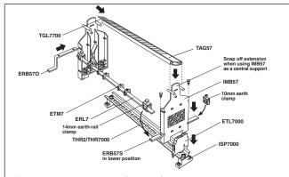
Figure 12: Mounting earthing and tagging accessories
