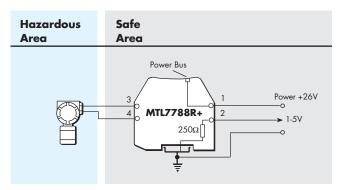
**Figure A2:** 2-wire transmitters with  $250\Omega$  conditioning
