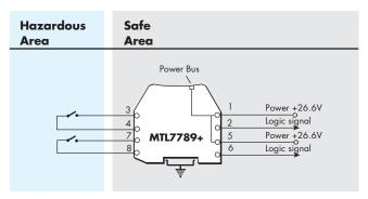
Figure A5: 2-channel switch inputs
