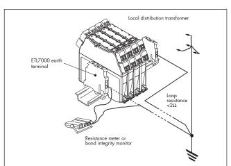
Figure 16: Earthing an installation with two conductors and providing resistance test facilities
