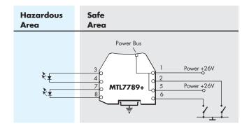
Figure A11: Low power digital outputs
