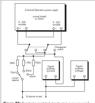
**Figure 23:** Constant-current test circuit using a power supply and digital multimeters
