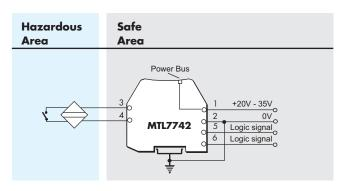
Figure A8: Single channel switch/proximity input
