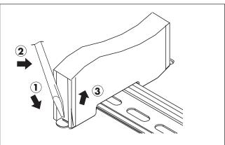
Figure 7: Removing an MTL7700 Series barrier from a DIN-rail
