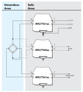
Figure A13: Strain-gauge bridges
