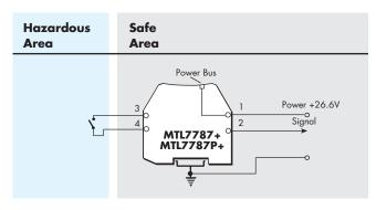
Figure A4: 2-wire transmitter/switch input
