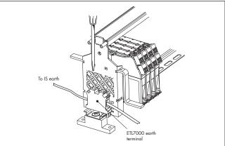
Figure 15: Plant earth connection to ETL7000 earth terminal
