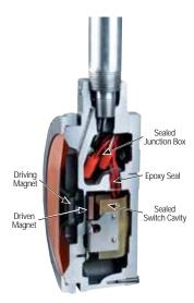
The Series P/G Ultra Mag™ Level Switch provides level indication by detecting pressure applied by the bulk material to the sensing diaphragm. The switch is tripped magnetically, as the result of 2 magnets with like poles repelling one another. The fields of the magnets perform through the nonferrous wall of the switch housing. Pins, links and "O" rings, which often cause failure due to moisture, dirt, and corrosion, are eliminated. The switch enclosure is completely sealed.
