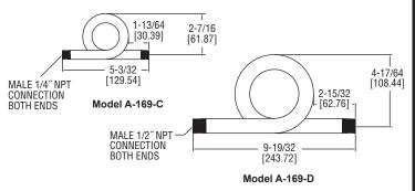
The **SERIES A-169** Carbon Steel Siphons protect pressure instruments in high temperature applications. Water held in the 180° coil prevents steam from contacting the instrument. Constructed with carbon steel, the A-169 siphons can withstand high temperature and pressure. They are ideal for use with pressure gages and instrumentation where the process media temperature exceeds the rating of the instrument. The male NPT connection allows for easy installation and secure attachment.
