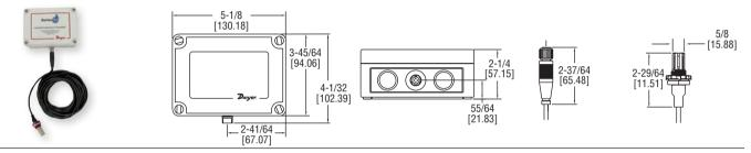
The SERIES RH-R Humidity Transmitter is the ideal transmitter for those applications where space is limited. The compact sensor is protected by a removable filter. It can be mounted up to 16 feet away from the weatherproof base. The Series RH-R is ideal for environmental chambers, rubber bladder burst detection and air handler applications.
