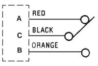
Pin Connections for Units with MS Receptacle
