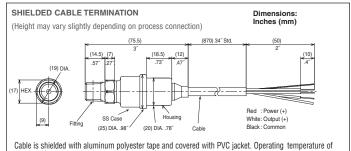
Cable is shielded with aluminum polyester tape and covered with PVC jacket. Operating temperature of  $-30/105^\circ\text{C}$ , storage temperature  $-40/120^\circ\text{C}$ . Cable includes drain wire. Vent tube provided in ranges of 300 psi and below. Individual wires are AWG 24 with tinned copper ends. Cable is rated at 300V, and is UL 2517 listed. 3 ft. (.9mm) standard length.
