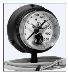
Indicating accuracy of Ashcroft Duragauge, above 300 psi with contact: Pointer not carrying contact – 1.0%. Pointer carrying contact – 1.5%. For ranges below 30 psi, add an additional ½% to indicating accuracies.
