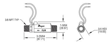
The SERIES P8 High Pressure Brass Flow Switches are ideal for high in-line pressures. Set points range from 0.25 to 2.0 GPM for liquid flow.
