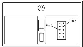
To apply the 1 Vdc signal to the MDI connect the precision voltage generator so that the positive line is connected to pin 7 and the ground is connected to Pin 6. **Step 13** The value displayed under the dashed line represents the as received reading for the 1 Vdc measurement. The reading will look as follows:
