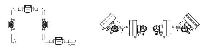
Figure 3: Installation positions
