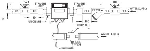
Figure 1: Installation diagram for TUF-150/400
