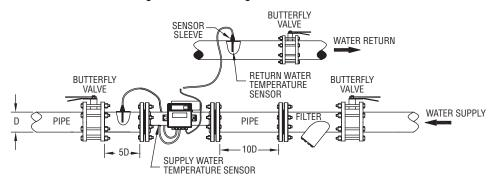
Figure 2: Installation diagram for TUF-500/2000
