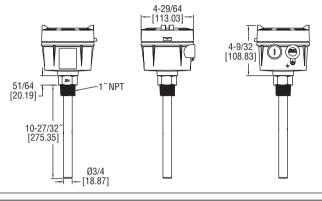
The MODEL VRLS Vibrating Rod Level Switches is economical choice in level detection of powders and bulk solids. The VRLS incorporates a piezoelectric crystal that vibrates the rod at its natural frequency, when contact material is present it dampens the vibrations and the switch changes state.
