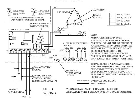
Wiring Diagrams for TD01-A to TD06-A: 110 VAC, TD01-B to TD06-B: 220 VAC, TD01-C to TD06-C: 24 VAC
