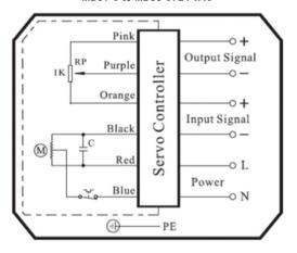
Note: To speed up installation of the control wires to the ACT-MDXX modulating actuator, it is recommended to remove the control module from the actuator. The control module can be removed by removing the two mounting screws on the left and right of the control module. Install the control wires to the correct terminal points and then reinstall the control module.
