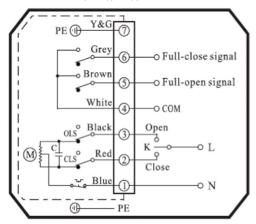
Wiring Diagrams for TD01-D to TD06-D: 24 VDC
