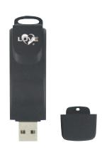
The Model MN-1 Mini-Node Communication Signal Converter is a low cost device that converts half duplex RS 485 serial communications signals into a signal that can be read by any computer with a USB port. The integral USB connector and RJ-45 connector reduces set up time by eliminating extra wiring. The Model MN-1 is powered via the USB connection which eliminates the need for an external power source. The compact size is great for field installation, control panels, and lab testing.
