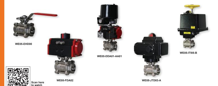
The SERIES WE05 offers the best possible design for socket weld ball valves. The swing out body feature and seat arrangement allow for trouble-free welding installation. The Series WE05 incorporates a full port 3-piece SS ball valve for ideal flow rates with minimal pressure drop. The valve features a blowout proof stem for added safety, reinforced PTFE seats and seals for longer life, and a 316 SS (ASTM CF8M) ball for better performance.
