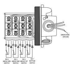
Figure 3: Wiring for factory sealed leads option. 1, 2, or 4 switches. Switch 1 wires are red, switch 2 wires are black, switch 3 wires are white, and switch 4 wires are brown. Wires are labeled C, NO, NC.
