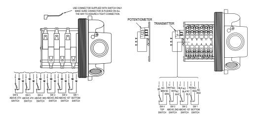
Figure 8: Wiring for switch types B, C, I, R, V, and W. 1, 2, 4, or 6 switches. Switch types B and I have "+" and "-" terminals.
