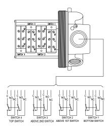
Figure 4: Wiring for switch type D. 1, 2, or 4 switches.
