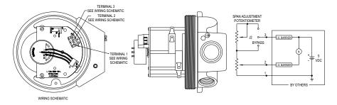
Figure 10: Intrinsically Safe wiring for potentiometer output. Refer to proper switch figure if unit has switches as well.
