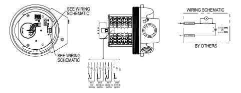
Figure 12: Intrinsically Safe wiring for transmitter with HART<sup>®</sup> communication output. Refer to proper switch figure if unit has switches as well.
