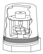
Models 19XXX, 39XXX and 49XXX Rotary Position Indicating Switches contain a 4-20 mA transmitter with HART<sup>®</sup> communication and two Single Pole Double Throw (SPDT) switches. Models 190XX, 390XX and 490XX contain a 4-20 mA transmitter with HART<sup>®</sup> communication only, no switches.
