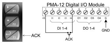
Figure 20. Acknowledge Relays w/Function Key or Digital Input
