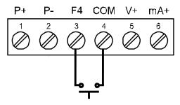
Figure 14. F4 Digital Input Connections
