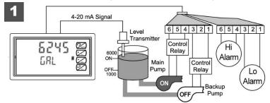
1. Relay #4 turns the main pump on at 6000 gallons and turns it off at 1000 gallons.
