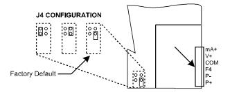
Figure 5. Transmitter Supply Voltage Selection
