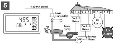
5. Relay #1 trips the Low Level Alarm at 495 gallons and resets at 750 gallons.
