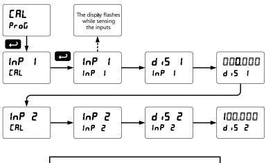
Warm up the meter for at least 15 minutes before performing calibration to ensure specified accuracy.
