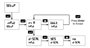
Set **d-SCAL** to no if both displays are to be used for anything other than PV1 & PV2.
