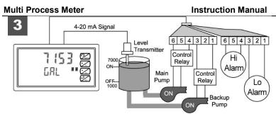
3. If the backup pump is not able to keep up, and the level reaches 7000 gallons, relay #4 transfers and starts the main pump as well.
