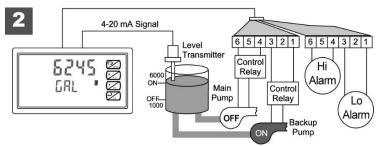
2. With the Pump Alternation feature activated, the next time the level reaches 6000 gallons, relay #3 transfers and starts the backup pump.
