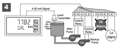
4. Relay #2 trips the High Level Alarm at 7500 gallons and resets at 6900 gallons.
