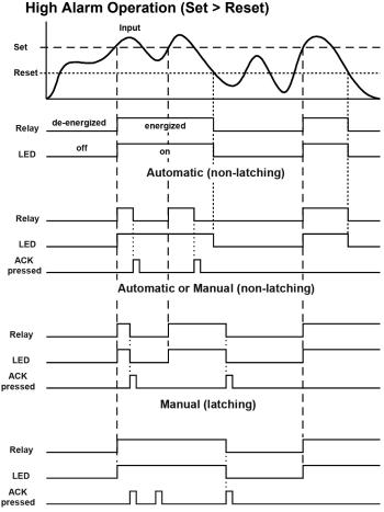
Manual only after passing below Reset (latching with clear)
