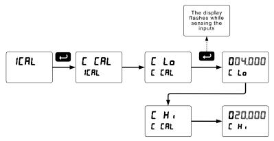
The graphic above shows the calibration of the current input. The voltage input is calibrated in a similar way.
