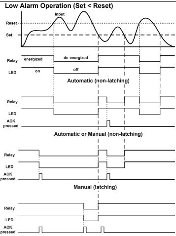
Manual only after passing above Reset (latching with clear)
