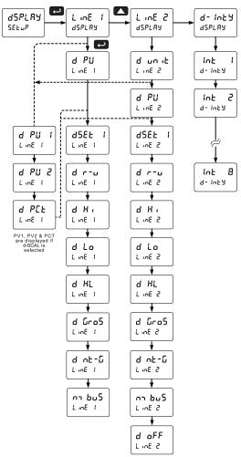
After setting up the input and display, press the Menu button to exit programming and skip the rest of the setup menu. Press the Menu button again and the Up arrow to reach the *Program* menu and complete the scaling or calibration of the meter.
