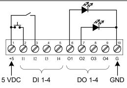
Figure 18. Digital I/O Module Connections
