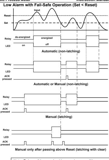
Note: Relay coil is energized in non-alarm condition. In case of power failure, relay will go to alarm state.
