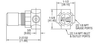
The SERIES MPR Miniature Pressure Regulators are compact units that provide low cost, high performance pressure regulation of compressed air or air/water. The low torque, non-rising adjustment knob with locking capability provides easy and precise adjustment. Models for use with air are self relieving. Models for air/water are nonrelieving.
